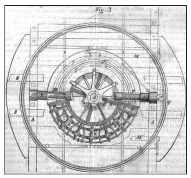
Figure 3.19. Robie's Balance Turn-Table. Plan View of Central Pivot Area. 1854. Note the width of the rail beneath the circular carriage atop the pivot is standard gauge (4 feet 8.5 inches).
