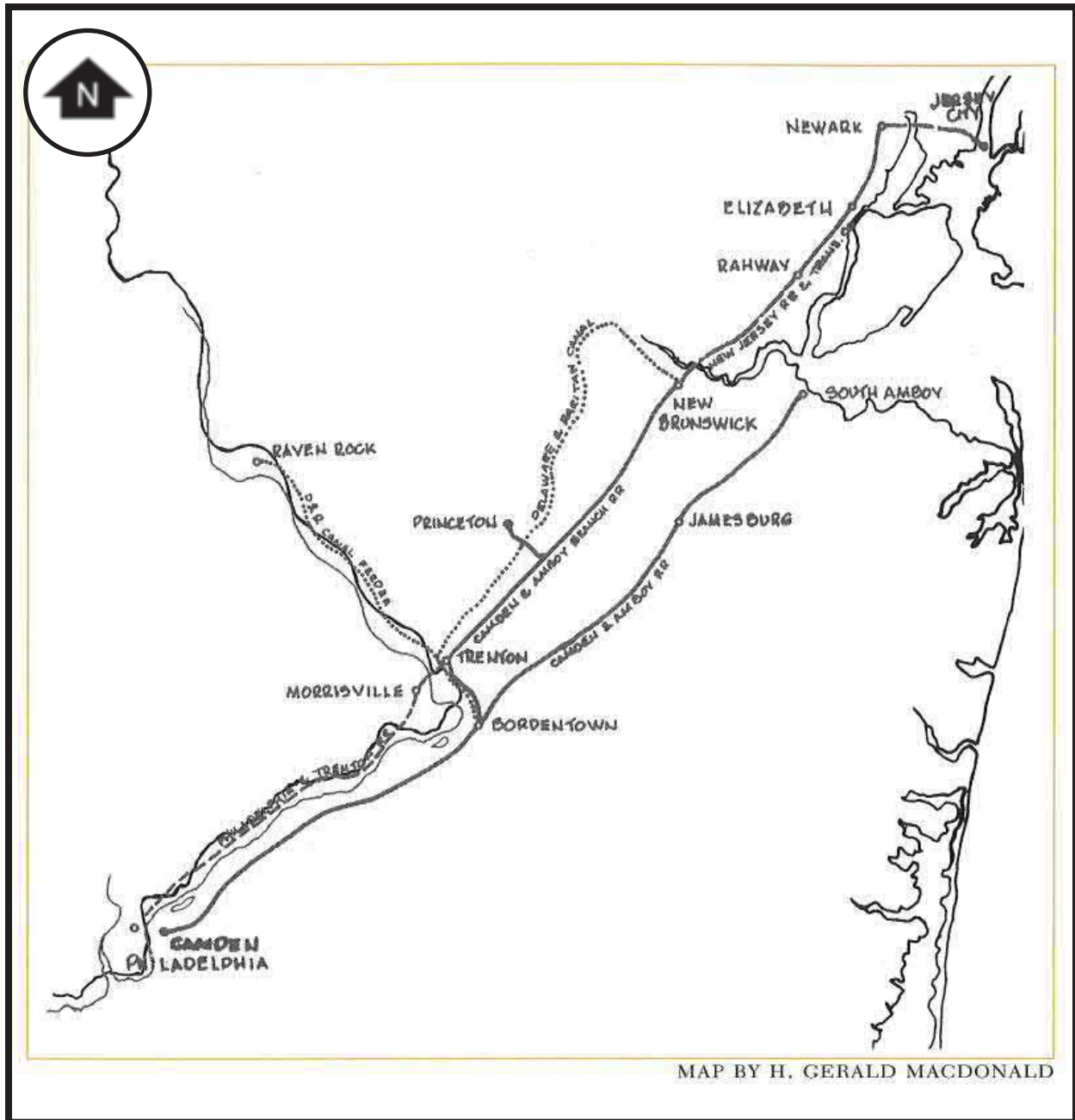
Figure 5.2. Camden and Amboy Railroad, circa 1839. The railroad's first section, completed in 1832, was between Bordentown and South Amboy. The second section, completed in 1834, was between Camden and Bordentown. A more logical all-rail route lay between Trenton and Jersey City, so a branch was built from Bordentown to Trenton in 1837 and extended from Trenton to New Brunswick in 1839. The New Jersey Railroad, a separately chartered company that would not be merged with the Camden and Amboy until 1867, completed the route between New Brunswick and Jersey City. Also shown are the route of the Delaware and Raritan Canal, operated with the Camden and Amboy Railroad as the Joint Companies, and the Philadelphia and Trenton Railroad, which offered service between those two cities and was operated by the Camden and Amboy Railroad beginning in 1836 (Source: Cunningham 1997).
