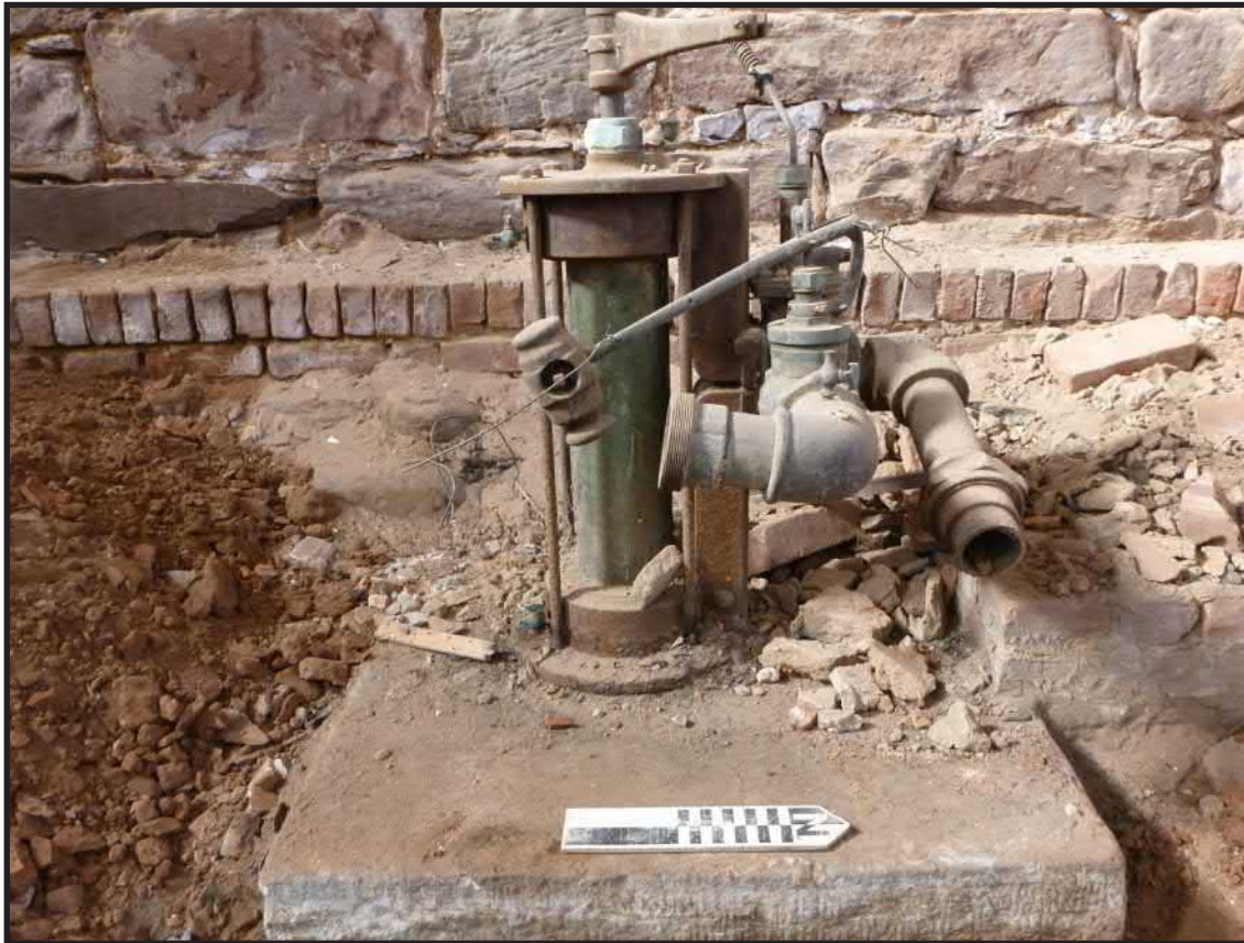
Photograph 3.5. Detailed view of the Ross Valve Manufacturing Company water engine uncovered in the crawlspace adjacent to the interior of the west wall of the church. Seated on a rectangular bluestone slab, this device was hooked up to the city water mains and used hydraulic pressure to power the bellows for the church's pipe organ. Note how the bluestone slab is mortared into the brick masonry at right, implying that the water engine was probably installed at the same time as the brick foundation. Scale in feet and tenths (Photographer: Joshua Butchko, January 2015) [HRI Neg. #15001/D2:035].
